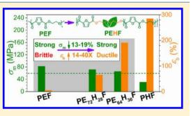
others are almost amorphous. In comparison with PEF, PEHFs with  $\phi_{\rm HF}$  of 28–36 mol % possess significantly improved tensile ductility (elongation at break 54–160%) and retain high tensile modulus (2.6–2.2 GPa) and yielding strength (71–65 MPa). The tensile properties are comparable to those of bottle-grade PET.
