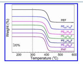
Figure 6. TGA curves of PEF, PHF, and PEHF copolyesters. (N<sub>2</sub>, 10  $^{\circ}$ C/min).
