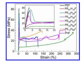
Figure 7. Typical stress-strain curves of PEF, PHF, and PEHF copolyesters.
