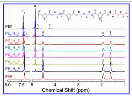
Figure 1. <sup>1</sup>H NMR spectra of PEF, PHF and PEHF copolyesters. Note: chemical shift at 11.6 ppm for solvent TFA-d<sub>1</sub>.
